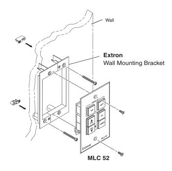
Mounting the MLC 52 to a mounting bracket (mud ring)
